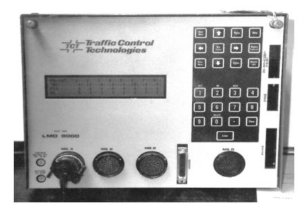
The settings in a modern traffic signal controller can be grouped into six timing categories:
