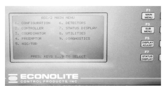
Basic settings include controller timings and functions required for isolated (non-coordinated) signal operation (initial, passage, maximum, yellow, all-red, recall, etc.) and rudimentary phase configuration information (phase rotation, start-up phases, flash entry and exit phases, etc).
